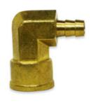
The BHFE Series is a Brass 90° Elbow, Female NPT threads to multi-barb Adapter. Available FNPT sizes are 1/8 inch, 1/4 inch, and 3/8 inch. Available barb sizes are 1/4 inch, 5/16 inch, 3/8 inch, and 1/2 inch. The temperature range is -40° F to 160° F. The maximum working pressure is 150 psi. This fitting is intended for use with a hose clamp.
