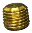
The BPC Series is a Brass recessed hex Plug with male NPT threads. The working pressure is 1200 psi and the temperature range is -65° F to 250° F. It is ASA, ASME and SAE compliant.
