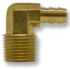
The BHME Series is a forged Brass multi-barbed  $90^{\circ}$  Elbow Adapter with male NPT threads. Available MNPT thread sizes range from 1/8 inch to 1 inch. In addition, available barb sizes range from 3/16 inches to 3/4 inches. Flow can be equal or reduced. The working temperature range is  $-40^{\circ}$  to  $160^{\circ}$  and the working pressure is 150 psi. Barstock is optional for some sizes (see list below).
