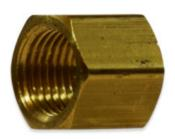
This Brass Cap has female NPT threads. The working pressure is 1200 psi and the temperature range is -65° F to 250° F.
