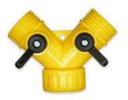
Garden Hose non-swiveling dual shutoff has a non-corrosive plastic body, ball and handle. It has a Zinc plated steel screw and Buna-N seal. It flows from female to male. Shutoffs are designed for city water pressure to a maximum of 80 psi. This valve does not swivel.
