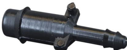
The VC-S Series are straight vacuum connectors in equal and reducing styles. It is made of Natural or Black Nylon 6/6. Equal barb sizes are 1/8 inch, 3/16 inch, 1/4 inch, 5/16 inch, 3/8 inch, 1/2 inch, and 5/8 inch. In addition, reducing barb sizes are 3/16 inch by 5/32 inch, 1/4 inch by 1/8 inch, 1/4 inch by 3/16 inch, 5/16 inch by 1/4 inch, and 3/8 inch by 1/4 inch. The working temperature range is -20° F to 212° F. These connectors are used for air, liquid, and vapor applications.
