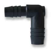
The L Series are standard triple-barbed elbow connectors and are offered in both equal and reducing sizes. These elbow connectors are molded of Natural Nylon or Polyethylene. Optional materials include: Natural and Black Polypropylene. Equal sizes are 1/4 inch, 5/16 inch, 3/8 inch, 1/2 inch, 5/8 inch, 3/4 inch, 1 inch, 1-1/4 inch, and 1-1/2 inch. Reducing sizes are 1/2 inch by 1/4 inch and 1/2 inch by 3/8 inch. Barbed fittings over 1 inch are not offered in Polyethylene.
