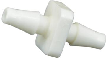
The C-SO Series are original single barbed straight and reducing connectors. These connectors have no parting line on the barb and have a square center hub. Also, tubing can be started on the barb of this connector before any expansion begins. It will expand the tubing by 43% when it is completely inserted. Available materials are Black and White Nylon, Natural Polypropylene, Clear Polycarbonate, and Natural PVDF. Available barb sizes are 1/16 inch, 3/32 inch, and 1/8 inch.
