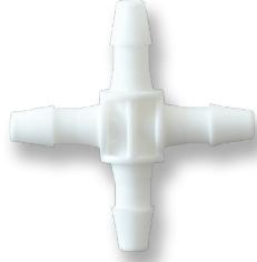
The CX Series is a standard single barbed Cross fitting with no molded parting line on the barb. The barb will expand the tubing to 50% above its normal size. It is available in White Nylon and Natural Polypropylene. The available equal barb sizes are 1/16 inch, 3/32 inch, and 1/8 inch. This cross-fitting is recommended for medical and laboratory environments.
