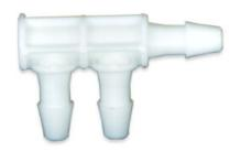
The DTF-S Series is a three-port F-style fitting usually used with flexible tubing. It can expand tubing by 50% of its normal ID. This permits high-pressure capabilities. This fitting is available in White Nylon and Natural Polypropylene. All three ports are equal. Available barb sizes are 1/16 inch, 3/32 inch, and 1/8 inch.
