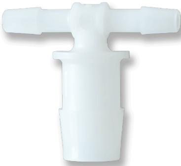
TR-R Series are standard single barbed reducing and enlarging tee connectors. Materials available are Natural and Black Nylon, Natural and Gray PVDF, Natural and White Polypropylene, Glass-Filled Black Nylon, and Polyethylene that is NSF 51/61 certified.
