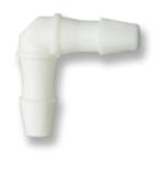
The EV Series are single barbed tube-to-tube elbows. These elbows are available in White and Black Nylon, Natural Polypropylene, Clear Polycarbonate, and PVDF. These elbows are available in equal or reduced sizes. Barb sizes are 1/16 inch, 1/8 inch, and 3/32 inch.
