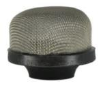
The RV Series inline Strainer filter is made of a flexible PVC housing with a 304 Stainless Steel 40 mesh screen (standard). Some sizes also have 20, 80, and 100 mesh screens available. This series comes in FNPT threads of 1/4 inch, 3/8 inch, 1/2 inch, 3/4 inch, and 1 inch. The maximum operating temperature is 160° F. Made for male pipe threads.
