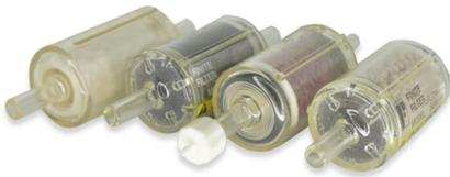
The IFF Series Nylon Filters come standard with 1/4-inch stems that accept tubing or push-in fittings to adapt to various configurations. Available with silica gel (SG) to remove moisture, activated charcoal (AC) to remove oil vapor, molecular sieve (13X) to remove hydrocarbons, or oil-activated dye (AO) to indicate oil. 1/8 inch barbs or 1/8, 3/32 inch elbows available.
