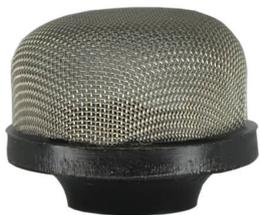
The RV Series inline Strainer filter is made of a flexible PVC housing with a 304 Stainless Steel 40 mesh screen (standard). Some sizes also have 20, 80, and 100 mesh screens available. This series comes in FNPT threads of 1/4 inch, 3/8 inch, 1/2 inch, 3/4 inch, and 1 inch. The maximum operating temperature is 160° F. Made for male pipe threads.
