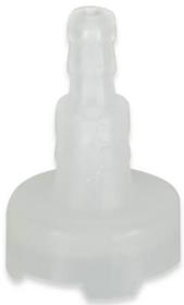
This Polypropylene Filter has a 3/16" hose barb connection with a 149-micron filter which is also Polypropylene. It can be used for any liquid container e.i. bottles and reservoirs. The feet prevent it from clogging by not sitting flush on any surface.
