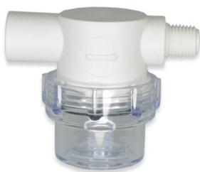
The PWF Series Plastic Bowl Filters have a Polypropylene or Nylon housing with a clear, profile 1-inch bowl filter. Available port sizes are 1/4 inch, 3/8 inch, and .170 inch barbs. Male and female NPT threads for these filters are 1/4 inch, 3/8 inch, and 1/2 inch. Available gaskets are EPDM, Viton®, and Buna-N. Filters: 20, 40, 80, 100, or 250 mesh 303 Stainless Steel; 5 and 70-micron Polyethylene screen; 10 Micron paper pleated screen.
