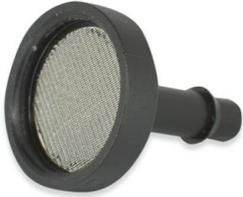
Pick-up filter for the end of tube lines. Barb fittings of 1/8", 3/16", 1/4", 5/16" and 3/8". Made of Polypropylene, Acetal, and PVDF with Polyester screens. The screens range from 10 microns to 250 microns. The screen is recessed at the bottom of the filter.
