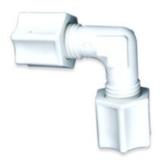
The CE Series Plastic Compression Elbow Fittings are used to allow a 90 degree tube connection without kinking attached tubing. Available in NSF approved Glass-Filled White Polypropylene, FDA and NSF approved Acetal (POM) for use with hot water applications, FDA and NSF approved Nylon, and UV resistant FDA and NSF rated PVDF. Provided with Poly gripper (except for 1/8 inch units) for us up to 220 psi.
