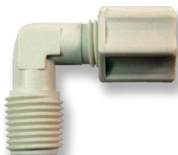
The CME Series are Male NPT Compression Fittings to an OD Elbow configuration. Use for Manifolds, Valves, Regulators, or mechanical instruments. They are molded of either Glass-Filled White polypropylene, NSF-approved FDA-approved Acetal for use with hot water applications, NSF-approved FDA-approved Nylon, or NSF-approved FDA-approved UV-resistant PVDF. Provided with a poly gripper for use up to 220 psi. 1/8-inch units do not have a poly gripper.
