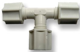
The CT Series Three port Compression Fittings are for a 1/8 inch to 7/8 inch tubing connection without kinking attached tubing. Available in NSF approved Glass-Filled White Polypropylene, FDA and NSF approved Acetal (POM) for use with hot water applications, FDA and NSF approved Nylon and UV resistant FDA and NSF-rated PVDF. Provided with Poly gripper (except for 1/8 inch units) for use up to 220 psi. Available in a select number of reducing sizes.
