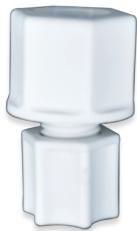
The CF Series Compression Female Pipe Threads, 1/8 inch to 1/2 inch, with compression fittings ranging from 1/4 inch to 5/8 inch tube connection without kinking attached tubing. Available in NSF approved Glass-Filled White Polypropylene, FDA and NSF approved Acetal (POM) for use with hot water applications, FDA and NSF approved Nylon and UV resistant FDA and NSF-rated PVDF. Provided with Poly gripper (except for 1/8 inch units) for us up to 220 psi.
