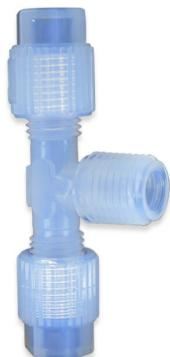
TGAT Series is a PFA compression Tee adapter with male NPT threads to two gripper rings. OD sizes range from 1/4" to 3/4", the male NPT threads range from 1/8" to 3/4".
