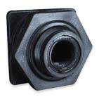
The BHF Series Bulkheads are made of Black Polypropylene ranging from  $\frac{1}{2}$  inch to 4-inch Female NPT sizes with 3/16 inch Santoprene Seals.
