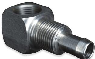
The EBHF Series is a tank flange 90° elbow Bulkhead. This series is available in Aluminum, Brass, and Stainless Steel. Female NPT thread sizes for this series are 1/4 inch, 3/8 inch, and 1/2 inch. Barb sizes for this series are 5/16 inch and 3/8 inch.
