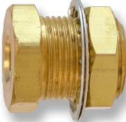
FBH Series inline Brass Bulkheads. FNPT both sides with exceptions, Elbow and several MNPT By FNPT. Brass Bulkhead sizes ranging from 1/8 inch FNPT thru 1 inch FNPT, Male to FNPT products are all 1/2 MNPT Dry seal located on the outside of the panel and FNPT on the inside of the panel, 1/4 or 3/8 FNPT. Zinc-Plated Steel optional,
