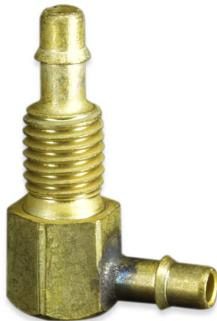
Brass Bulkheads with Bite-Style Barbs. 10-32 inch UNF mounting Threads for 1/16 inch, .078 inch, and 3/32 inch. 1/4-28 inch mounting Thread with 1/16 inch thru hole to 5/32 inch Barb. 5/16-24 inch mounting Thread with a 1/16 inch thru hole to 3/16 inch Barb. 3/8-24 inch mounting Thread with a 1/16 inch thru hole to 3/8 inch Barb. Mixed sizes are available for Straight and Elbow models.
