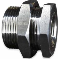
The LSSB Series are 316 Stainless Steel Bulkheads, available in sizes ranging from 1/8 inch, 1/4 inch, 3/8 inch, and 1/2 inch FNPT. The maximum working pressure for these bulkheads is 150 psi and the working temperature range is -4°F to 356°F. For larger sizes with gasket options please see our [\*\*BLSS series\*\*](#).
