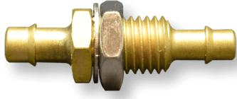
Brass Bulkheads with Bite-Style Barbs. 10-32 mounting Threads for 1/16 inch, .078, and 3/32 inch. 1/4-28 mounting Thread with 1/16 inch thru hole to 5/32 inch Barb. 5/16-24 mounting Thread with 1/16 inch thru hole to 3/16 inch Barb. 3/8-24 mounting Thread with 1/16 inch thru-hole to 3/8 inch Barb. Mixed sizes are available for Straight and Elbow models.
