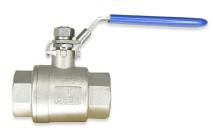
This two-way Brass Ball Valve has a pressure rating of 600 psi, and 150 psi is the working steam pressure. The maximum temperature is 366°F. The stem is blow-out proof, the ball is Chrome-plated Brass and the seat is PTFE. There is an adjustable screw packing nut. Both ports are equal in size and female NPT threads.
