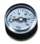
This Pressure Gauge has an ABS case with a Brass movement and a dial size of 1". The Gauge is available in 30, 60, 100 and 160 psi. There is a 1/8" MNPT center back mount that can also accommodate a 10-32 male UNF fitting inside that 1/8" fitting. The operating temperature for this gauge is 0° F to 160° F. The maximum supply is 50% over the gauge pressure range. This gauge is recommended for use with steam, air, oil and water.
