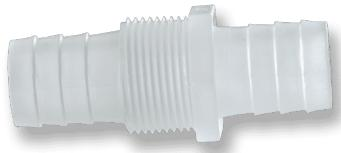
BHUC is a 1/2 Barbed bulkhead with an 11/16-24 Thread for the panel mount. 18 MM hole for the mounting through hole. Molded in several materials: Acetal, PVDF, and Polypropylene. Rated at 50 PSI. This bulkhead comes with a nickel-plated nut or with an Acetal nut.
